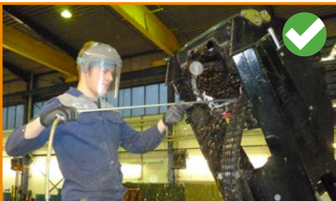
Cleaning boom system with high pressure air compressor!
